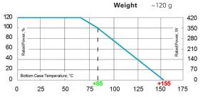
Derating (thermal resist.) UXP®-350: 5 W/K (0.2 K/W) Power rating: 350 W at 85°C bottom case temperature\*
